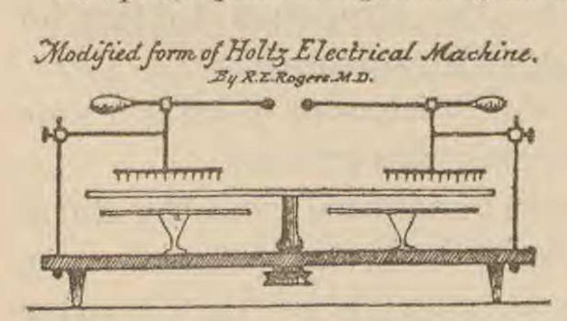
or upon removable rubber standards. The rotating plate is made to rotate horizontally over them, its axis passing vertically downward through the table, the driving wheel being underneath. Two standards carry the combs, etc., and can be swung round out of the way. Every part of the machine can be removed in a charged state, to be tested and compared with its
